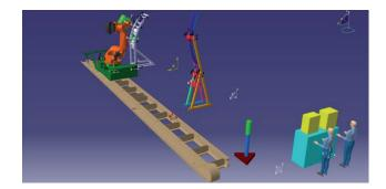
Robot Calibration Work Cell Layout showing test stand positions, robot on the rail, and tracker position.
