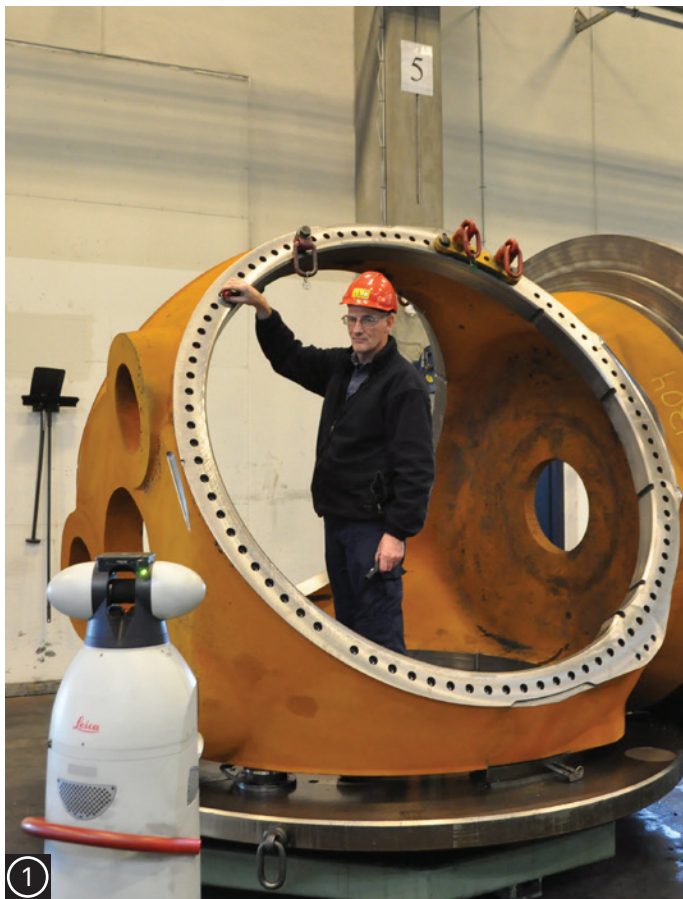
① Measuring a hub is a one man job with the Leica Absolute Tracker AT901. ② Up to 200 measurement points are relevant on a wind turbine hub. ③ PowerLock automatically connects the laser beam to the reflector.
